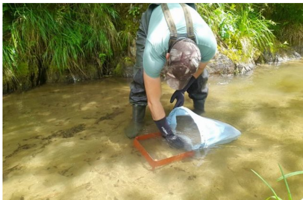
Sampling for aquatic macroinvertebrates using a Surber sampler. Photo: Foundation Conservation
